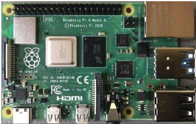
Figure 4. Photo of Raspberry Pi 4 2018
